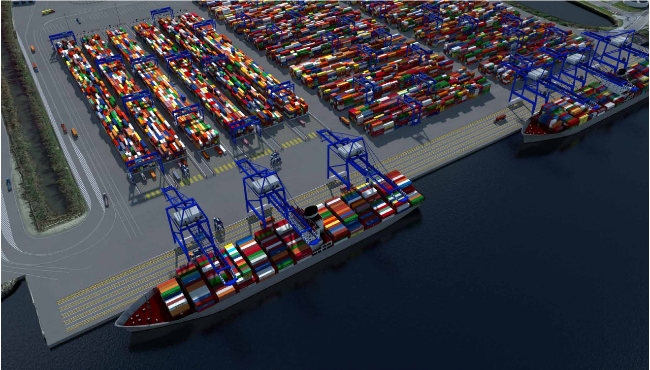
FIGURE 3. Visualisation of a container terminal converting van RTG + TT to ASC + ShC in a hybrid operation
